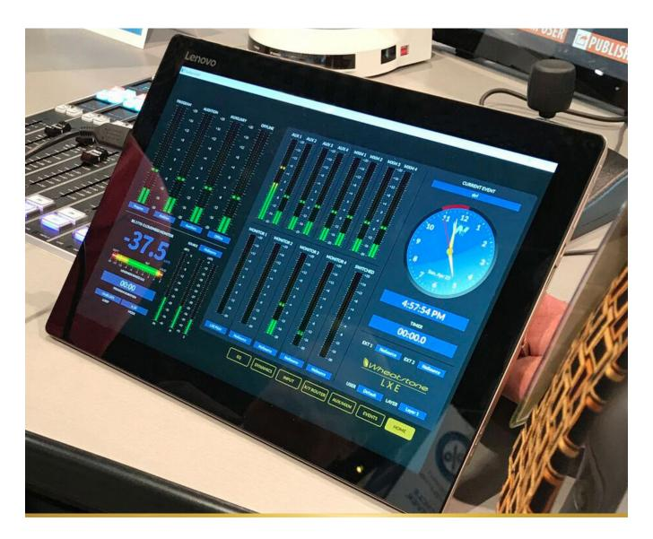
Not only can audio programming today function in a console-free environment, it can be more tightly routed and integrated with program automation systems, such as RCS Zetta, Enco, and BSI through IP.
